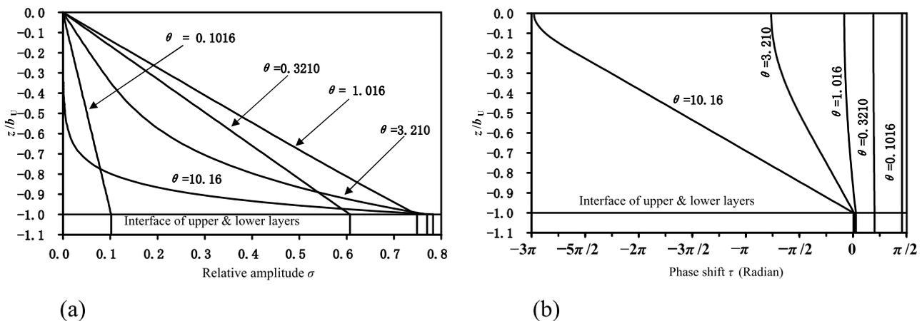
**Figure 5.** Changes of (a) relative amplitude  $\sigma$  and (b) phase shift  $\tau$  of sinusoidal air pressure fluctuation in the upper layer with the dimensionless elevation  $z/b_U$  for different values of air-leaking-resistance parameter  $\theta$  when  $d = 1.266$  and  $r = 0.1$ .
