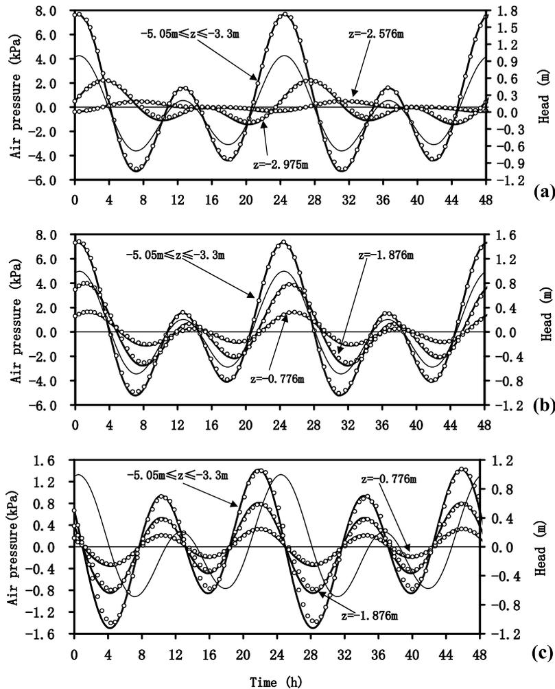
**Figure 3.** Changes of air pressures with time at different depths in the unsaturated zone above the water table for two-component head  $H_p(t)$  given by Table 3 when the air permeability of the upper layer equals (a)  $10^{-16} \text{ m}^2$ , (b)  $10^{-14} \text{ m}^2$ , and (c)  $10^{-12} \text{ m}^2$ . Thick curves, analytical solution (5a); circles, numerical solution to original nonlinear model; thin solid curves, head  $H_p(t)$ .
