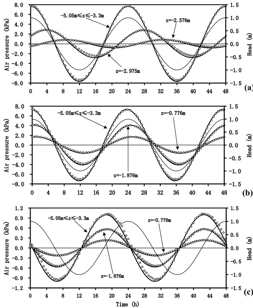
**Figure 2.** Changes of air pressures with time at different depths in the unsaturated zone above the water table for single-component head  $H_p(t)$  given by Table 2 when the air permeability of the upper layer equals (a)  $10^{-16} \text{ m}^2$ , (b)  $10^{-14} \text{ m}^2$ , and (c)  $10^{-12} \text{ m}^2$ . Thick curves, analytical solution (5a); circles, numerical solution to original nonlinear model; thin curves, head  $H_p(t)$ .
