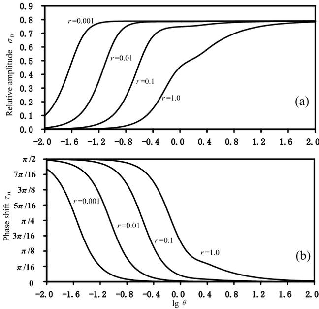
**Figure 4.** Changes of (a) relative amplitude  $\sigma_0$  and (b) phase shift  $\tau_0$  of sinusoidal air pressure fluctuation at the bottom of the upper layer ( $z = -b_U$ ) with the air-leaking-resistance parameter  $\theta$  for different values of  $r$  when  $d = 1.266$ .
