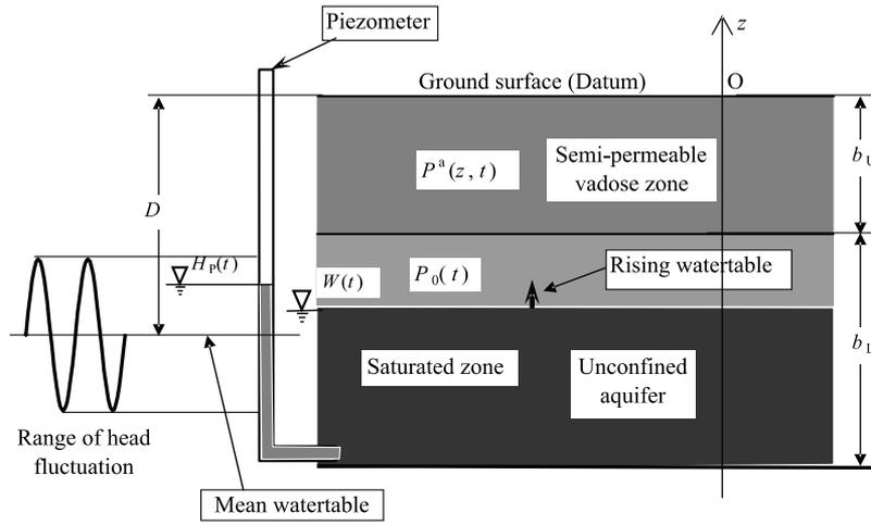
**Figure 1.** Schematic of airflow induced by fluctuating water table.
