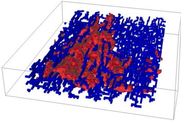
**Figure 1.** Portion of a 3D dendritic network where conduits occupy 9% of the volume showing an isoconcentration surface. Mass is transported preferentially in conduits. Diffusion and slow advection occur in the matrix. Flow is in the viewing direction.
