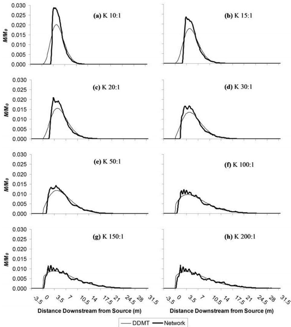
**Figure 4.** One-dimensional integrated mass distribution profiles of the PFP network and equivalent DDMT plumes at different PFP/matrix conductivity contrasts in the base case. Simulation time is 0.13 pore volume.
