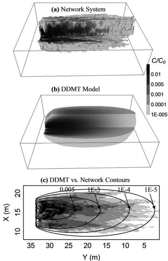
**Figure 2.** Comparison of plume matches by the DDMT model at a conductivity contrast of 100:1 in the base case: (a) 3-D network plume, (b) equivalent DDMT plume, and (c) 2-D network versus DDMT contours. Fill contours represent the true network model; line contours represent the DDMT model. The 2-D contours are vertically averaged from the original 3-D plume snapshots at time 0.13 pore volume.
