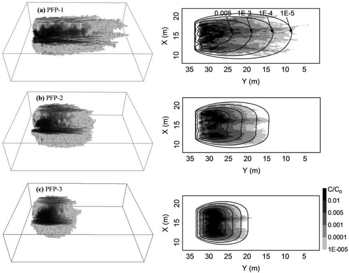
**Figure 5.** Plume comparison among different PFP network realizations at a constant PFP/matrix conductivity contrast of 50:1. Simulation time is 0.13 pore volume. The calculated mass transfer rate coefficient in the DDMT model is  $9.0 \times 10^{-4} \text{ d}^{-1}$  in realization 1,  $15.4 \times 10^{-4} \text{ d}^{-1}$  in realization 2, and  $27.6 \times 10^{-4} \text{ d}^{-1}$  in realization 3.
