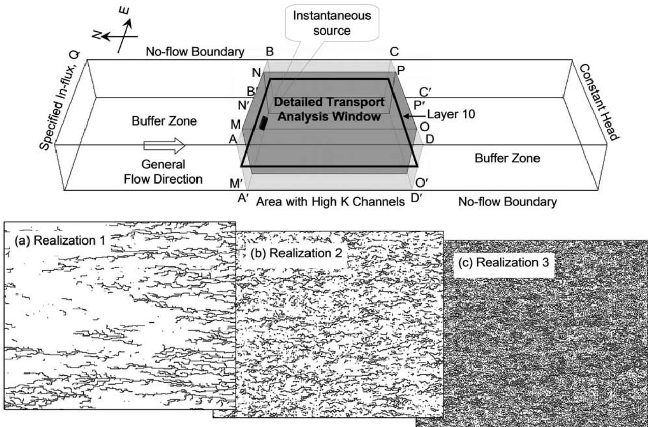
**Figure 1.** Schematic diagram of 3-D synthetic-aquifer model. Also shown are the PFP images at layer 10 of the detailed transport analysis window: (a) PFP network realization 1, (b) PFP network realization 2, and (c) PFP network realization 3. The volumetric fraction of PFPs is  $\sim 9\%$  in realization 1,  $\sim 20\%$  in realization 2, and  $\sim 46\%$  in realization 3.
