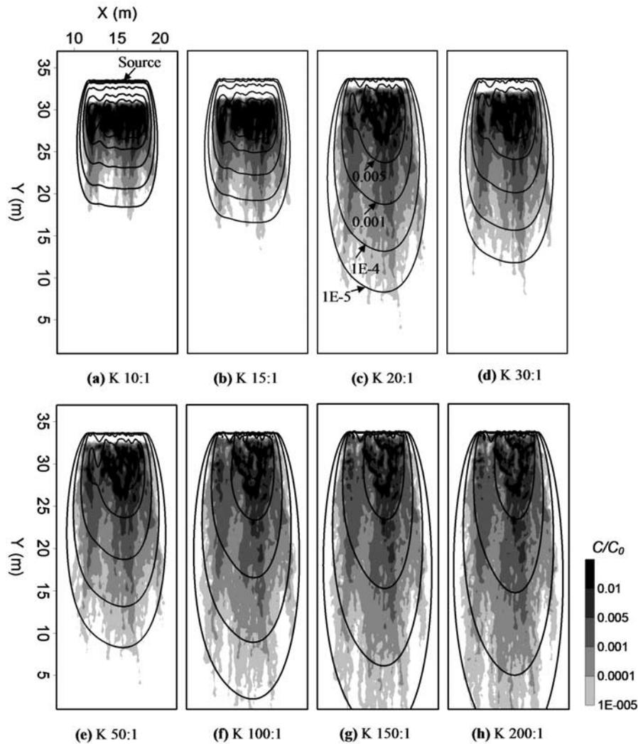
**Figure 3.** Plume matches by the DDMT model at different PFP/matrix conductivity contrasts in the base case. Simulation time is 0.13 pore volume. The calculated *RMSE* for each conductivity contrast is presented in Table 3.
