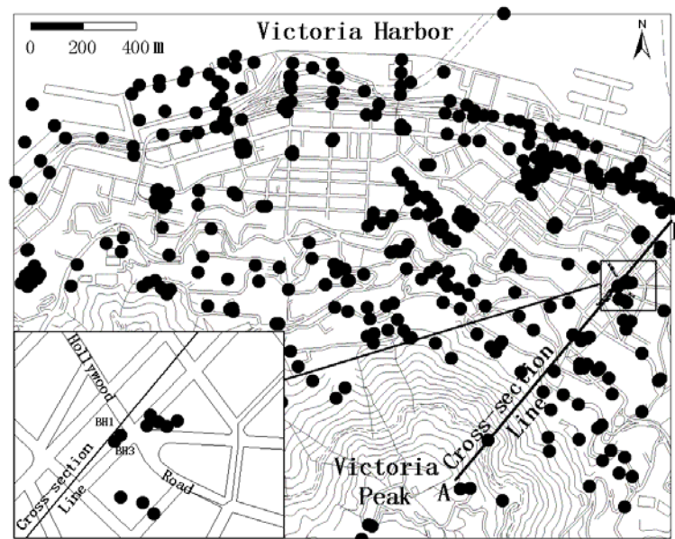
Figure 1: Location of BH1 and BH3 at No. 52, Hollywood Road, Sheung Wan, Hong Kong. Hundreds of boreholes (black dots) were installed in this area based on which 3D geological models can be constructed.
