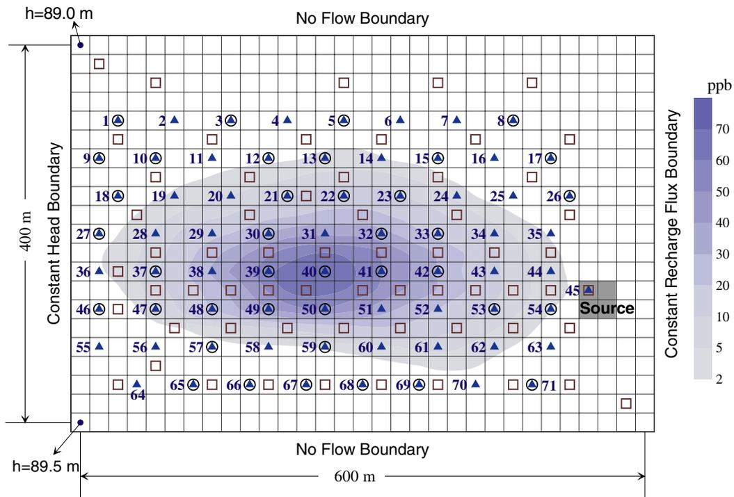
Fig. 2. Configuration of the monitoring network design problem. The solid triangles indicate the pre-defined potential monitoring well locations. The open circles denote the optimal monitoring wells selected by NGA. The color-filled contour map represents the concentration distribution at the end of the monitoring period output by the transport model for the hydraulic conductivity field kriged using 62 known  $K$  values (shown as open squares).
