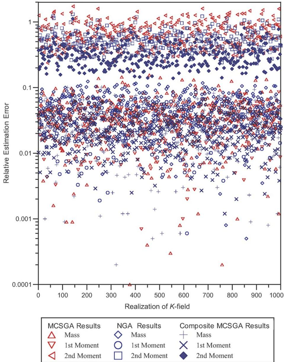
Fig. 4. Comparison of relative estimation errors of global mass and higher moments for 1000 realizations of the *K*-field under different network design methodologies. The errors are computed as the relative differences between the plume interpolated from the optimal monitoring wells and that given by the transport model without any interpolation for 1000 conditional realizations of the *K*-field.
